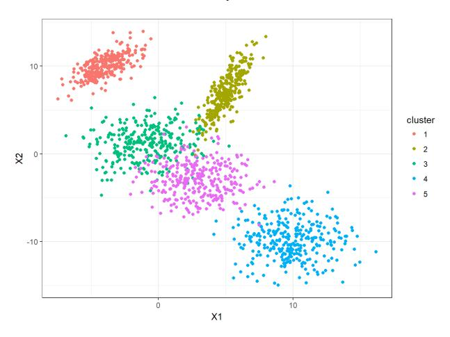
The results of running a k-means clustering algorithm, which is a commonly-used unsupervised learning algorithm. The machine has grouped the points into different color-coded, unnamed categories based on their proximity to each other. This image is taken from Thean Lim's explanation of k-means clustering.
